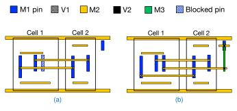
(a) pin access failure; (b) pin access success. [Xu+,DAC'14]
