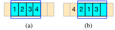
Fig. 3: Example of local reordering with sliding window. (a) Sliding window at one step; (b) next step.
